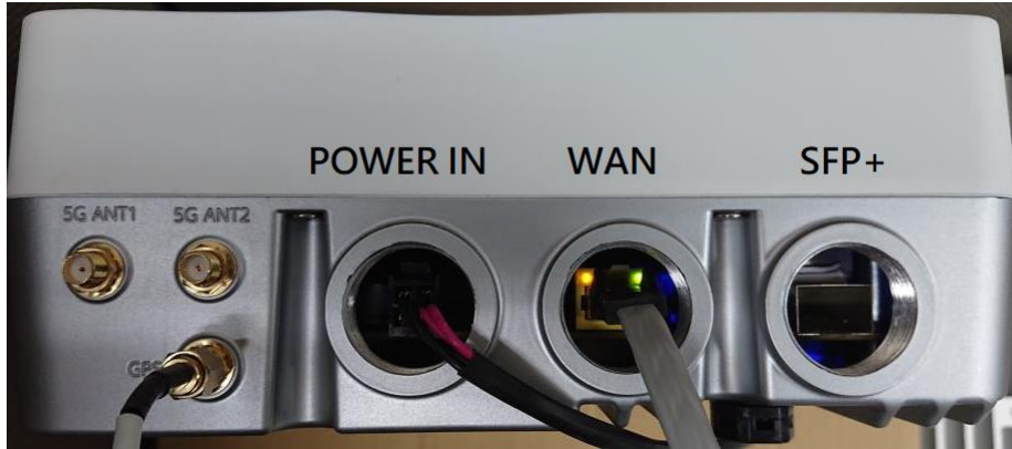
Figure 2. The Network Interfaces of the Askey 5G NR Small Cell (SCU2140)
