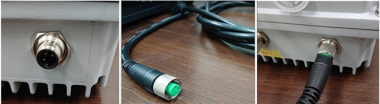
Figure 8. Power cable installation diagram
