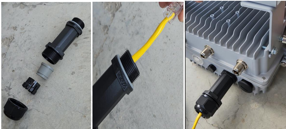
Figure 9. Network cable installation diagram
